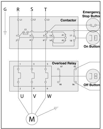
Figure 90. G0588 3-phase wiring diagram.
